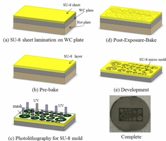
Fig.4 Fabrication process of SU-8 micro mold.
