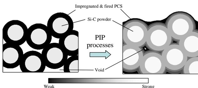
Fig. 8 Schematic of PCS-derived Si-C ceramics specimens before and after multiple PIP processes.
