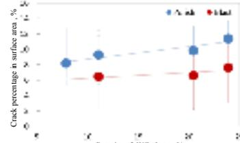
Porosity of WC plates vs. crack percentage in surface area
