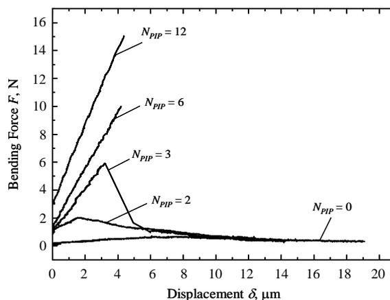
**Fig. 3** Bending force-displacement relations.
