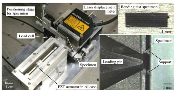
**Fig. 2** Three-point bending test apparatus.
