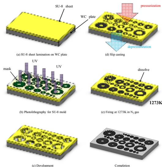
Process flow for fabricating microscale SiC ceramics parts.
