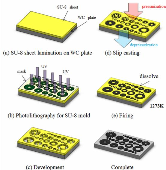
Fig.2 Fabrication process of SiC-MEMS ceramics parts.
