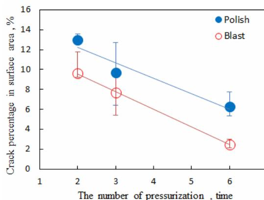
Fig. 7 Relationship between the number of pressurization and the ratio of crack using WC plate with the porosity of 11.1%.
