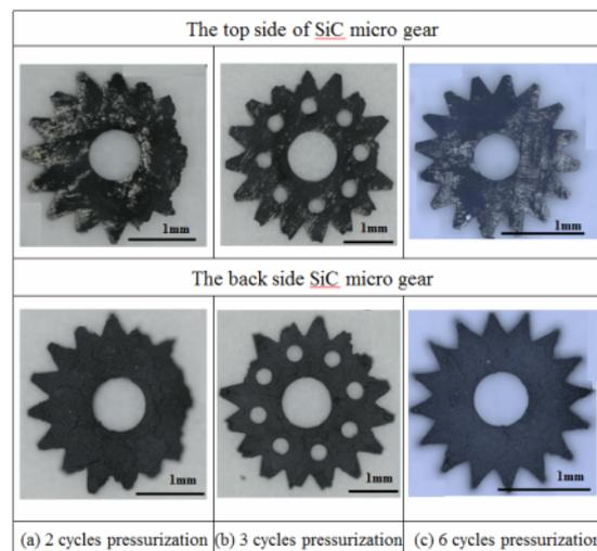
Fig. 6 SiC micro gears fabricated by micro slip casting using WC plate with the porosity of 7.9%.
