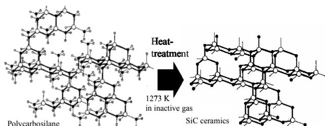
Fig.1 Construction model of PCS precursor for SiC.
