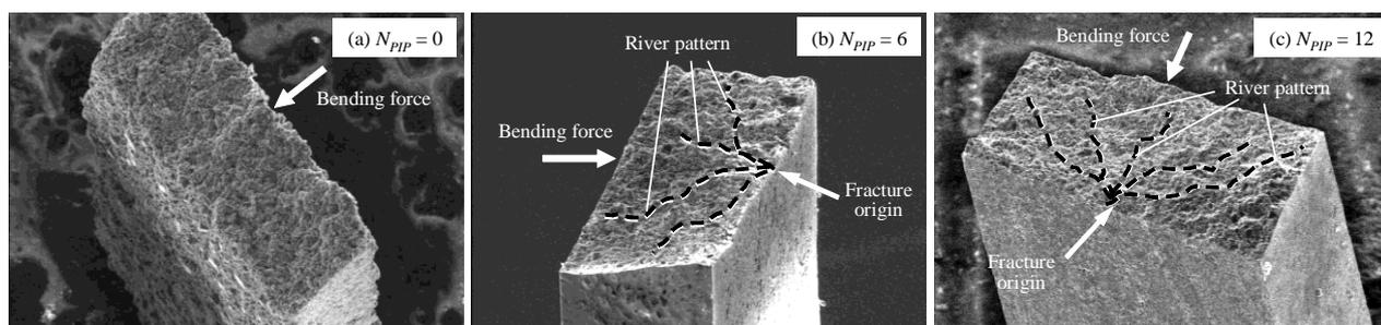
Fig. 7 SEM photographs of fracture surface of PCS-derived Si-C ceramics.
