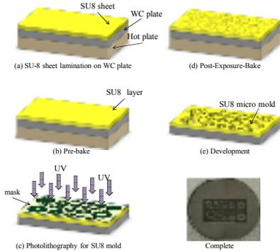
Process flow for fabricating SU8 micro mold.
