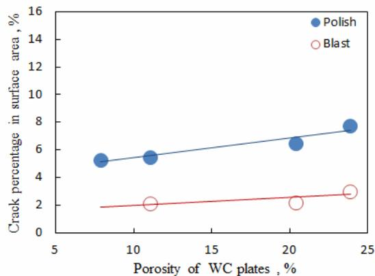
Fig. 8 Relationship between WC plate porosity and crack percentage at 6 cycles pressurizations.
