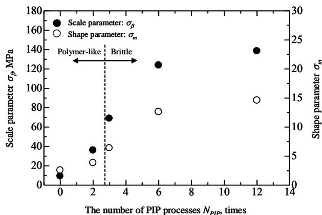
**Fig. 6** Relationship between the number of PIP process and Weibull parameters.
