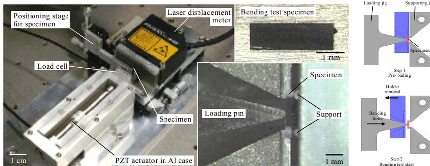
Specially developed three-point bending tester for miniature Si-C ceramics along with a schematic of testing procedure.
