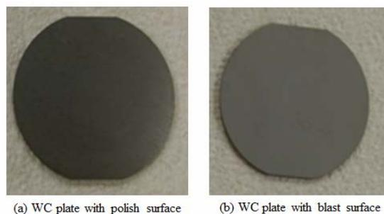
Fig.3 Porous WC plate with the porosity of 11.1%
