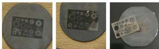
(a) Fine (b) Partly delamination (c) Delamination
