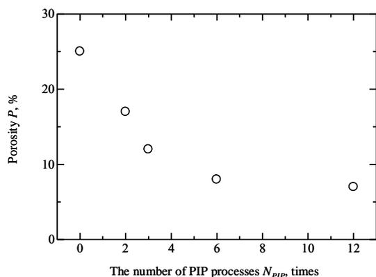
**Fig. 1** The number of PIP process vs. porosity.
