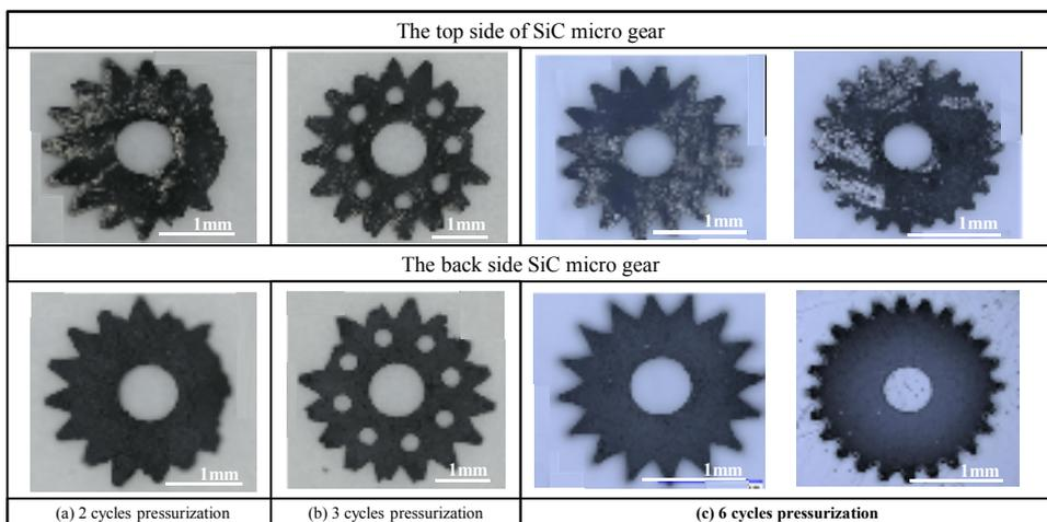
SiC micro gears fabricated by micro slip casting using WC plate with porosity of 11.1%.
