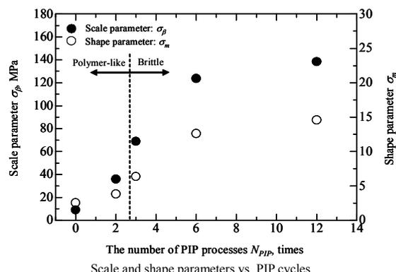
Scale and shape parameters vs. PIP cycles.
