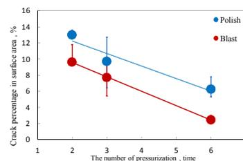
The number of pressurization vs. crack percentage in surface area
